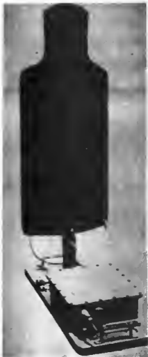
Figure 84 Automatic target device (M31A1) with E-type silhouette
